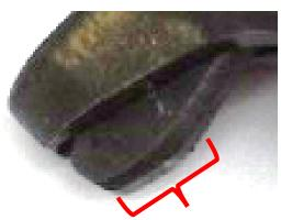
This may especially be the case with worn or imprecisely made grip frames in which the retaining shoulder is insufficient to correctly position the *magazine catch*.
