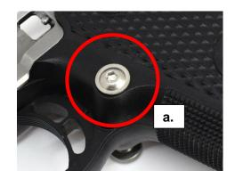
b. Apply Loctite 243 (blue) or a comparable, non-permanent thread locker to the grub screw. Using a long Allen key with a spherical head position it through the opening in the back of the grip frame and tighten it in the cross piece until noticeable resistance can be felt. The cup point of the grub screw shall engage the material of the grip frame to ensure safe retention of the *magazine* catch.
