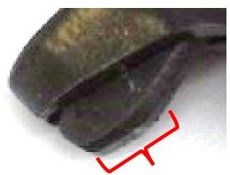
This may especially be the case with worn or cheaply made, unprecise grip frames in which the retaining shoulder is insufficient to correctly position the *magazine catch*.
