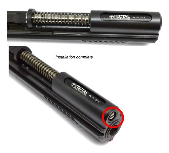
3. The correct tightening of the guide rod shall be checked regularly. The front end of the guide rod shall always be located behind the muzzle (see above pic.).
