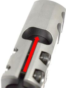
2. Adjust / rotate the *muzzle brake* to its proper orientation and lightly tighten the clamping bolts.
